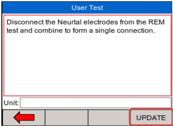
In case the user test requires data entry such as a result, the user test can also include an engineer unit such as Ohms, Watts, Celsius etc. Confirm the entry by pressing the UPDATE button. Once the test sequence is completed, press the back arrow key and confirm the changes:
