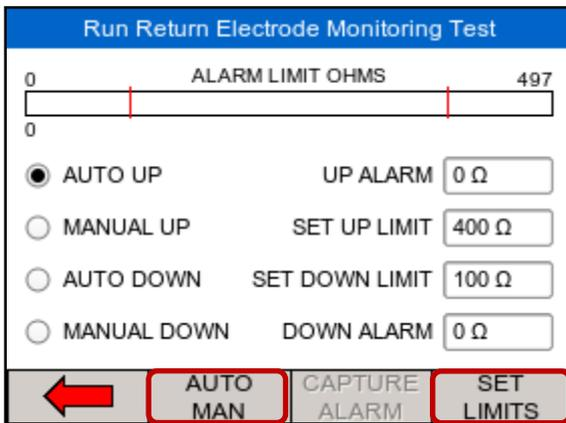
Select automatic (up or down) or manual (up or down) control by using the dedicated AUTO MAN key. This key is also used to set the limits. Once the SET LIMITS field is highlighted in green, use and press the rotary encoder to manipulate the UP and DOWN limits.
