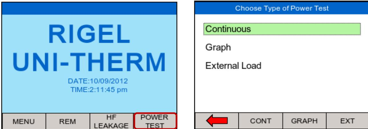
Select Power test from the home screen; then select F2 (CONT) F3 (GRAPH) or F4 (EXT) modes using the fast keys; to select either the Continuous, Graph or External Load test. Use the rotary encoder or the dedicated function keys to navigate.
