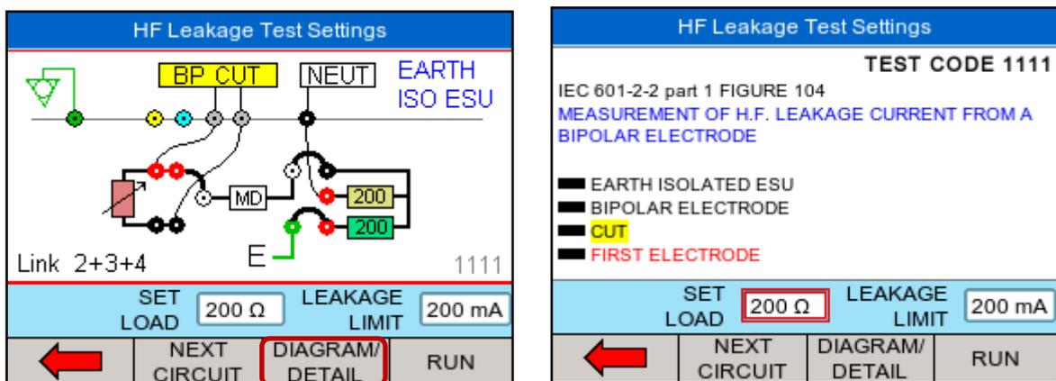
The rotary encoder can be used to scroll the different test setups, or to SET LOAD and LEAKAGE LIMIT values. The selected field is highlighted in red. Press the rotary encoder to activate the field (field turn blue) and use the rotary encoder to change the settings. Press the rotary encoder again to confirm
