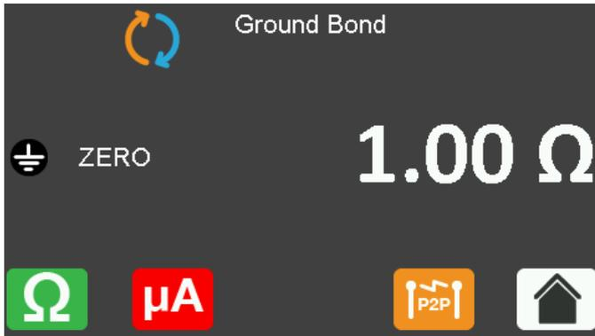
The SafeTest 50 will automatically start the test when it is selected and will automatically stop by pressing the **Leakage**, Point To Point or Home icon.
