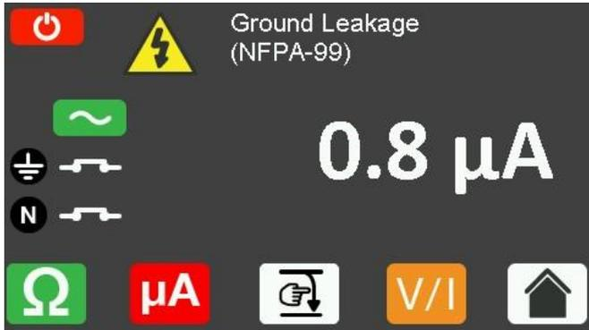
To apply mains voltage in Normal Polarity and START the test, press the
