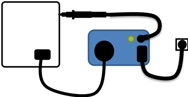
**Note:** Each time the ground bond probe is placed on a new test point, the zap circuit will be reactivated, ensuring accurate readings at every measurement point.
