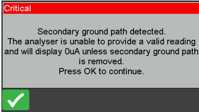
To perform a valid test, the secondary ground must be removed. Testing with a secondary ground will lead to invalid readings as the leakage current will flow through the low resistance secondary ground rather than the high resistance (1kΩ) [body model](#) in the SafeTest 50.
