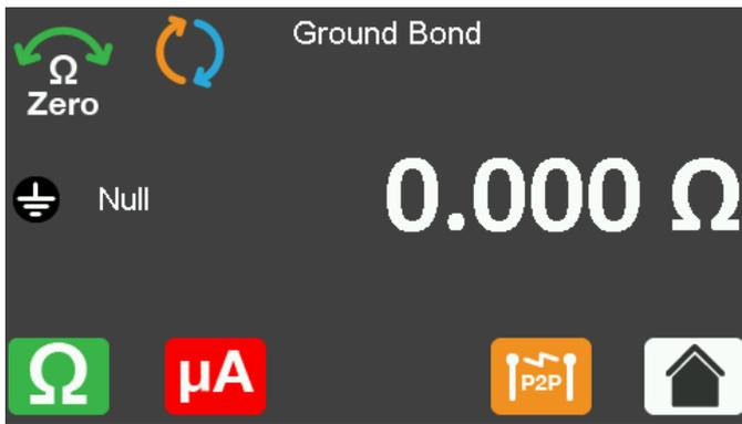
To remove the lead compensation, remove the probe and press the
