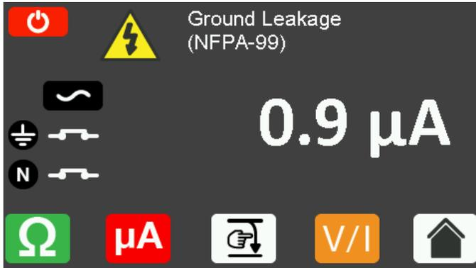
To apply mains voltage in Normal Polarity and Start the test, press the
