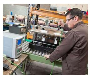
This forms an integral part of the quality control processes at the factory, which produces over 3000 machines a year, and enables the company to undertake fast and accurate electrical safety and run testing without damaging product.
