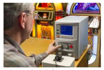
The HAL 101 enables Sound Leisure to undertake fast and accurate electrical safety testing without damaging the product under test, capturing important data and completing testing in line with the relevant compliance and product testing standards.
