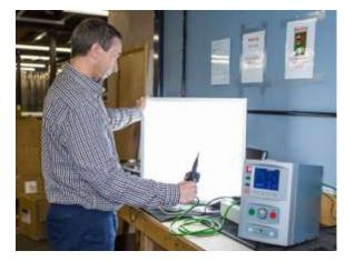
continuity and ground/earth bond tests alongside AC/DC Hipot (FLASH/Dielectric Strength) to ensure JCC's products guarantee product quality, performance and reliability and are safety compliant with EN 60598. This covers the safety of fixed lighting equipment such as recessed and surface luminaires.
