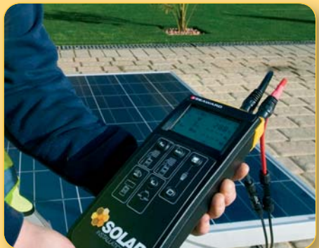
Figure 20. The Seaward PV150 Photovoltaic Tester measures and stores data for verifying PV electrical system integrity and performance.
