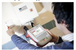
Fixed equipment or appliances are more difficult to inspect and test due to their connection to the fixed wiring of an installation. This does not mean that only visual inspections are required for these types of equipment and they should be subjected to a full combined inspection and test intervals determined by risk assessment.
