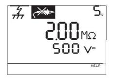
If an external connection e.g. a probe is required, the display will flash the connection icon. The user needs to connect the probe. The test can then proceed when the Green or Enter button is pressed. At the end of each test in the test sequence, the display will indicate the result.
