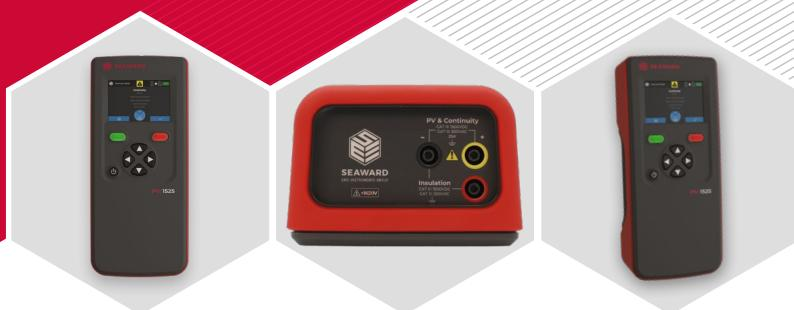
**The PV:1525 is designed for installers and O&M engineers to allow electrical safety testing and performance measures in PV systems up to 1500 V<sub>DC</sub> and 25 A<sub>DC</sub>, which is ideal for residential and commercial level installations.**
