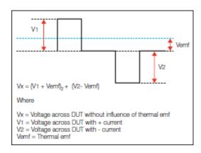
Measurement of joint resistance of 2 busbars
