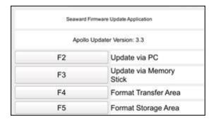
Press F2 to Update via PC (Apollo+ Series). Connect the USB lead between the PC and the Apollo+ Series and press F1, as instructed.
