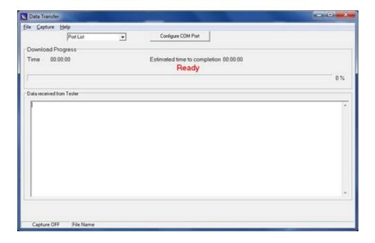
4. Using the drop down Port List, select the correct COM Port as earlier identified. Then click Configure COM Port. The following screen will be displayed, dependant upon the use of a USB Serial connection one of the
