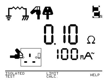
3. Connect the earth bond probe to an earthed point close to mains socket which the EUT is plugged. This can be the screw head of the mains socket housing or the earth pin of an adjacent socket.
