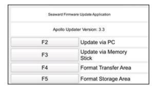
Press F2 to Update via PC (Apollo+ Series). Connect the USB lead between the PC and the Apollo+ Series and press F1, as instructed.
