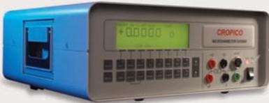
The Cropico DO5000 microhmeter is the ideal instrument for cable testing; it has the automatic temperature compensation required with the flexibility to set both the cable material's exact temperature coefficient and the temperature which the measurements are referenced to. In addition the DO5000 can operate with a continuous measurement current or a single current pulse. Switched DC measurement mode can also be set.
