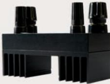
A four terminal resistance standard is constructed with 2 current terminals connected to the ends of the resistance element and 2 potential points connected at the adjusted value of the standard. This method of construction ensures repeatable values to be achieved when connecting to the standard's terminals.
