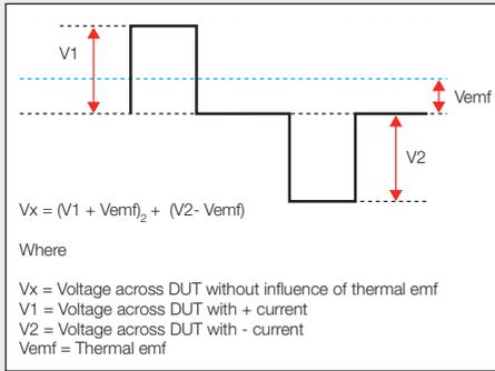
The second method sometimes employed is to connect the current terminals of the ohmmeter together, and with the potential leads connected to the DUT, measure any thermal emf that may be present. This measured value is then stored and deducted from the next measurement with current and potential leads connected to the DUT in the normal way. This is all done automatically when using Crocico Ohmmeters in the auto zero mode.
