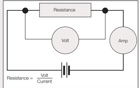
There exists a variety of resistance measuring instruments that will calculate and display the resistance reading without the need for calculations by the user. These measuring instruments will employ either a two wire or a four wire measurement technique.
