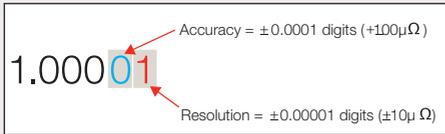
A measured value can also be displayed with a very high resolution but low accuracy i.e.  $1\Omega$  measured to an accuracy of 1% but a resolution of  $100\mu\Omega$  would be displayed as  $1.0001\Omega$ . The only meaningful digits would be 1.0100, the last two digits only showing the fluctuations in the measured values. These fluctuations can be misleading and emphasising any instability of the DUT. A suitable resolution should be selected to ensure a comfortable reading of the display.
