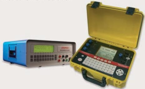
The Cropico Ohmmeter type DO5000 has all the facilities required to measure the temperature rise of machines.
