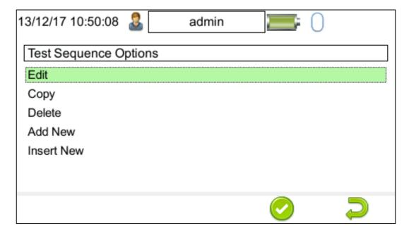
Select **Add New** using the keyboard arrow keys and the **Accept** button **Sequence** to the bottom of the test sequence list.
