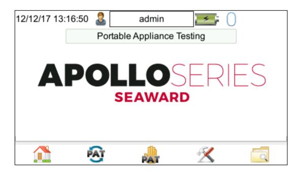
In the **Portable Appliance Testing** window select the **Tools** function **Settings** window.
