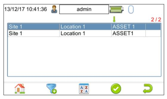
This is the Accept function, use the keyboard arrow keys to highlight an asset and use F4 view any corresponding results.
