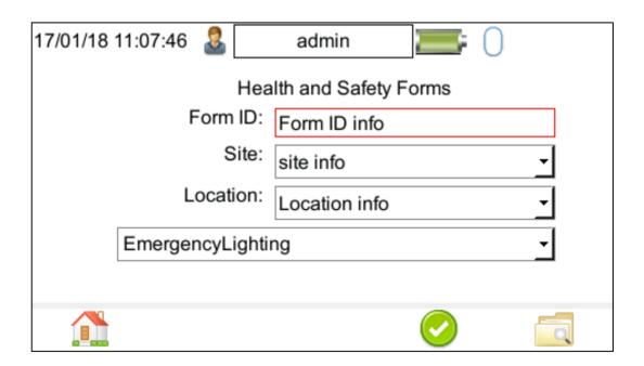
Enter a **Form ID**, the **Site / Location** information and the form required – **EmergencyLighting** from the dropdown and use the **Accept** button (F4).
