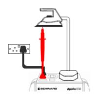
This test is applicable on Class I and Class II Equipment.
