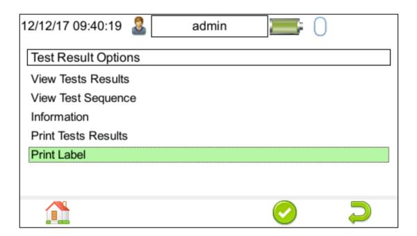
In the **Test Result Options** window, highlight and select **Print Label** using the **Accept** function to a selection window and displays a virtual representation of the label.
