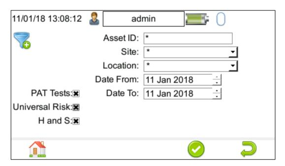
Note: If filtering the data, select the filters you wish to apply using the keyboard arrow keys and when complete press **Accept** using (F4).
