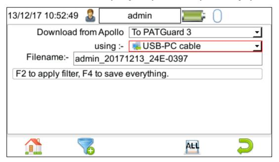
In the **Download from Apollo** field select **To PATGuard 3**, using the keyboard arrow keys to select from the dropdown menu.
