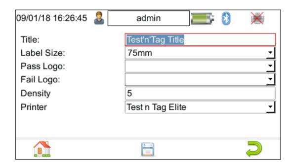
Using the keyboard arrow keys, highlight the bottom field for **Printer** and, from the dropdown, select the Bluetooth printer you paired earlier (**Note**: This will add / remove fields depending upon the selection made).
