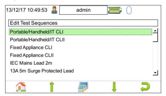
Altering **Test Sequences**: with a sequence highlighted, press the menu button (F3) to open the **Test Sequence Options** menu.
