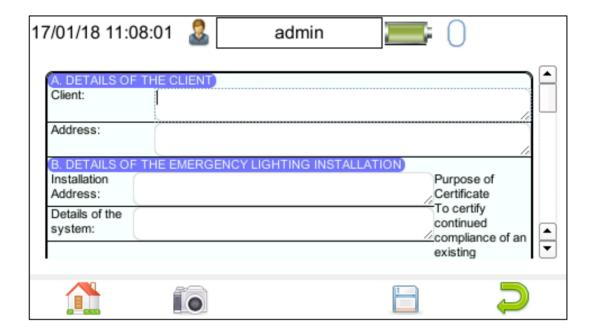
Use the keyboard arrow keys to move through the form and the QWERTY keyboard to complete the relevant fields.
