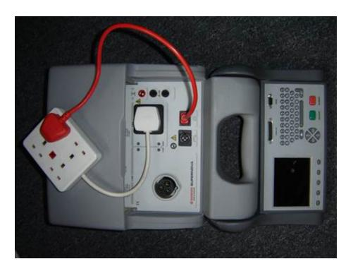
Both the Supernova and Europa Plus portable appliance testers come with 17 Factory programmed test sequences. It is not possible to add any extra sequences to this list, therefore in order to add this sequence one of the existing sequences must be sacrificed, ideally one that is not used.
