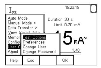
The following screen will appear, ensure the tester is set to Failure Menu within the On Test Failure section.
