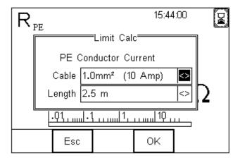
By pressing the OK button the pass value is now updated and the test can be performed.
