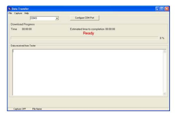
Ensure you have selected the correct COM Port, this will be the same port used for downloading of test results. You can check the port settings by clicking Configure COM Port. A display will appear, ensure your settings are set as below. If not change them and confirm by pressing Apply, then OK.
