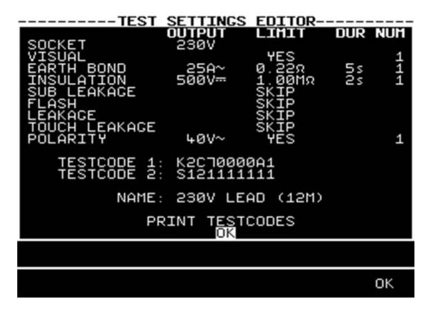
This screen shows the sequence of tests to be performed. In the example above it has been decided to alter the 12m 230V lead test.
